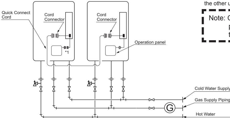
\*1 When connecting two units, disconnect the operation panel connector from the other unit.
