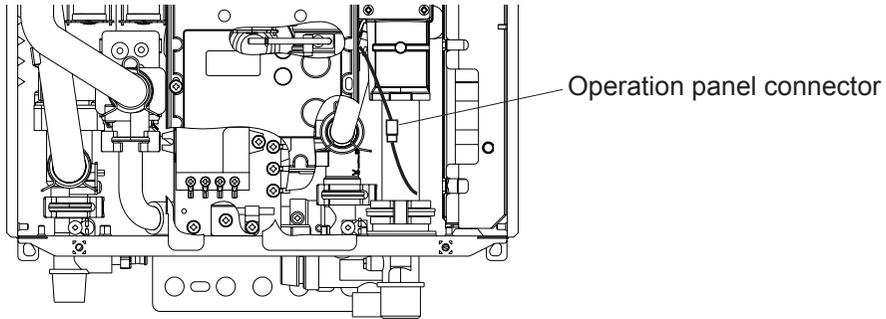
3. Cut off the connector at the end of the operation panel wires and the Y-shaped terminals (two-cord) of remote controller cord.
