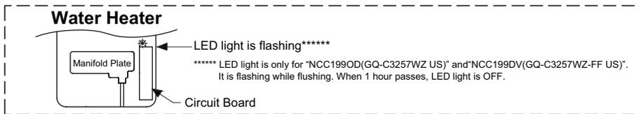
6. When 1 hour passes, the code “C00” is flashing on the Remote Controller. **C00** Flashing
