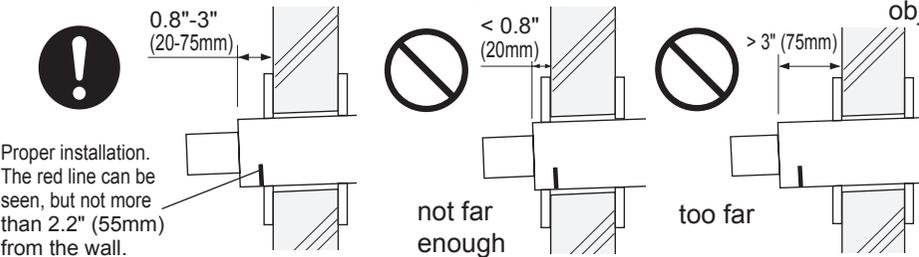
Proper installation. The red line can be seen, but not more than 2.2" (55mm) from the wall.
